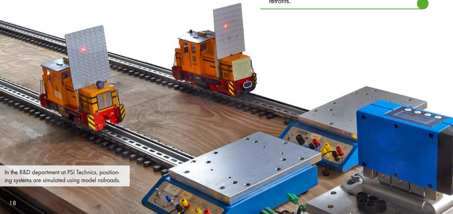
In the R&D department at PSI Technics, positioning systems are simulated using model railroads.
