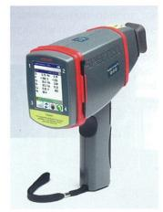
less accessible. The instrument incorporates an exclusive SPECTRO ICAL system for convenient one-sample, onetime calibration. Its simplified software features an intuitive touchscreen interface with two menu levels.
