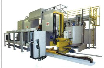
ing furnace, two austenitizing, carburizing and carbonitriding bell furnaces, with a working temperature up to 1,050 °C, a quenching oil tank max. 100 °C, a tempering furnace under N2 atmosphere, a washing machine with two tanks, a storage are about 500 mm diameter, 700 mm height for a surface of 0.19 m<sup>2</sup>, a volume of 0.155 m<sup>3</sup> and a maximum weight of a load about 300 kg.
