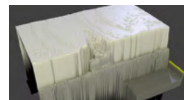
Center right: Elevation map created by a laser line scanner Lower right: 3D rendering of the recorded data
