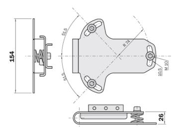
Figure 9: Mounting the TPCC
