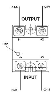
Figure 18: Connecting the Solid-state Relay
