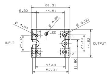
Figure 19: Installing the Solid-state Relay
