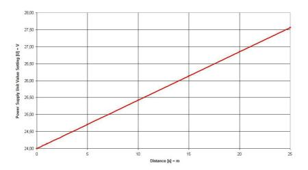
Figure 21: Line Drop,  $2.5mm^2$  Cable Cross-Section
