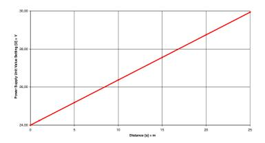
Figure 20: Line Drop,  $1.5mm^2$  Cable Cross-Section
