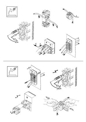
Figure 15: Cable Feeds and Frame Installation Overview
