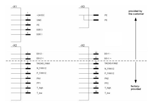
Figure 17: Terminal Board Pin Allocation
