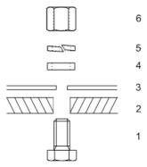
Figure 10: Mounting the TPCC Using Clearance Holes
